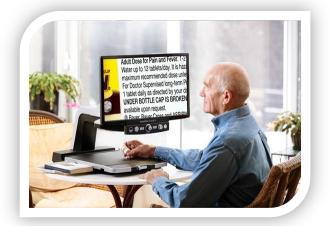
The other accessible station has a SARA reader and SmartView Synergy CCTV unit and is on a table that can be raised and lowered. The SARA station can scan and read a book to an individual in one of 18 languages, and patrons have the ability to change the reading speed and volume. The SmartView Synergy CCTV is designed for people with macular degeneration, diabetic retinopathy or other low vision eye conditions as it can enlarge the text.
