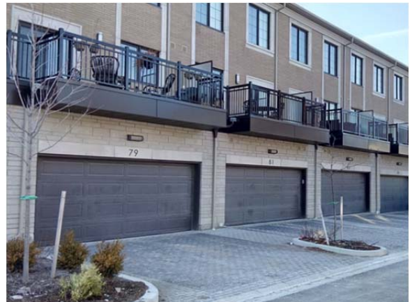
Image: Example of enhanced treatment of laneways with landscaping elements including tree planting using structural soil and permeable pavers.
