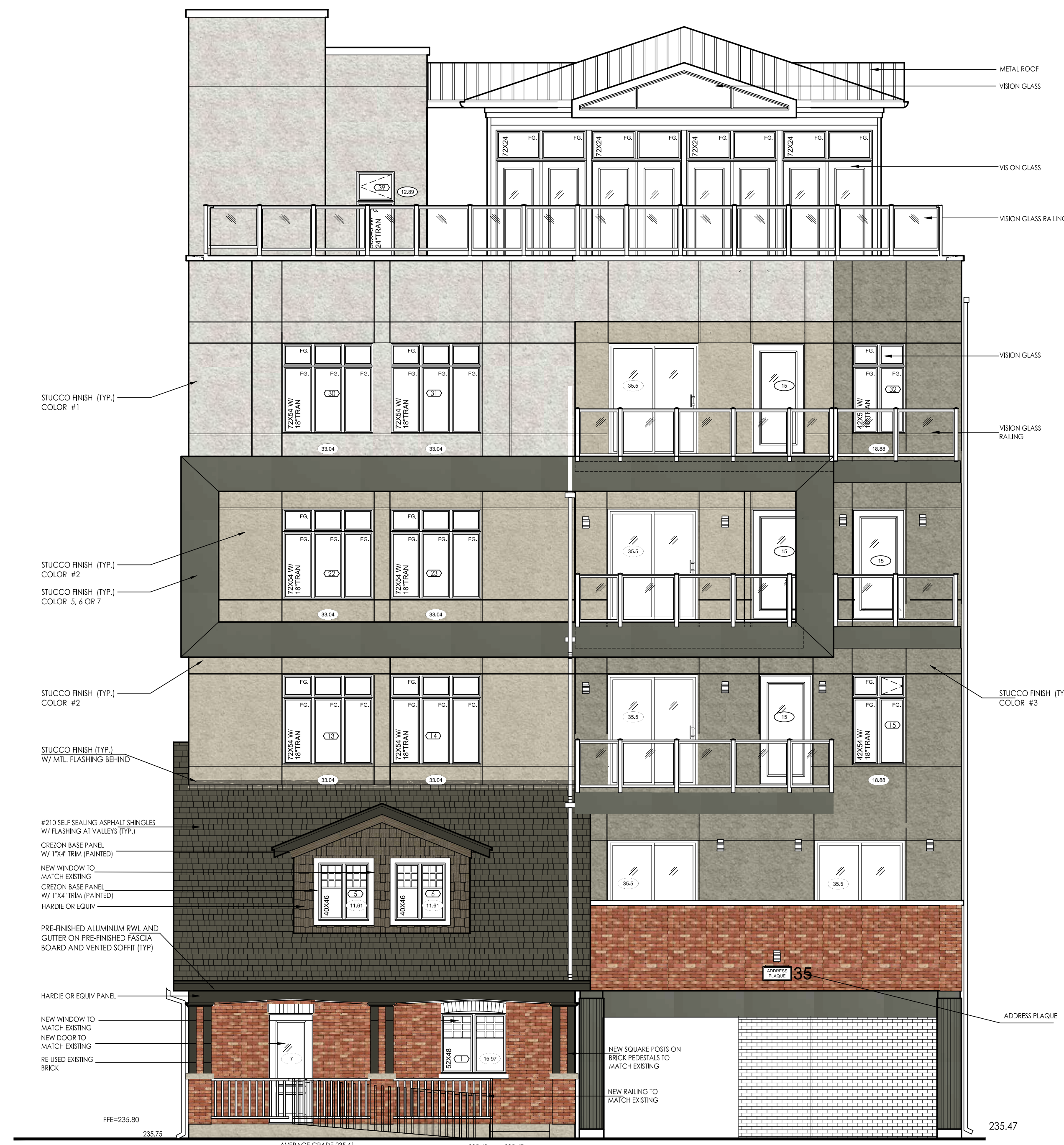
FRONT ELEVATION 5 STOREY
