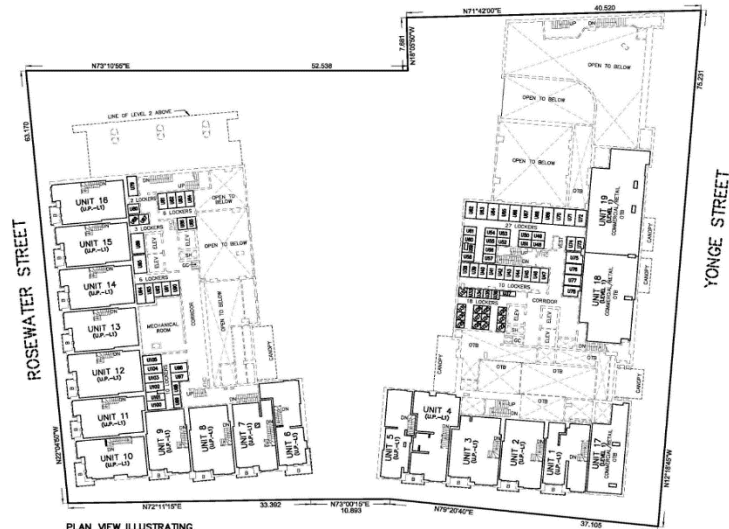
PLAN VIEW ILLUSTRATING UNITS 20 TO 105 INCLUSIVE (Storage), LEVEL 1 (Mezzanine) UPPER PORTION OF UNITS 1 TO 16 INCLUSIVE (Residential, Townhouse Units) AND
