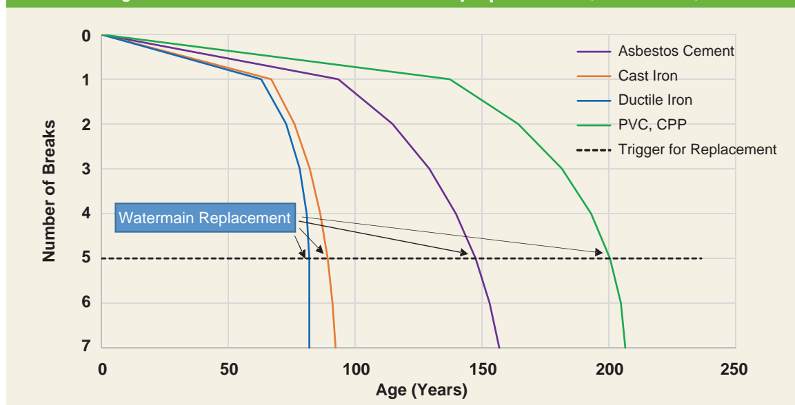
Figure 58: Estimated Deterioration Curves by Pipe Material (Watermain)
