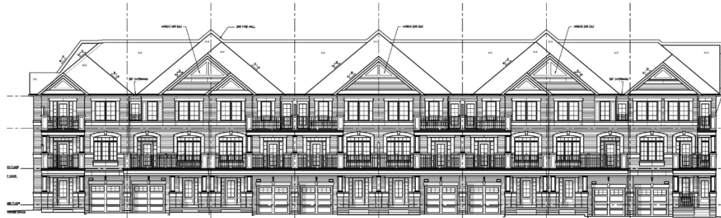
FRONT ELEVATION (TYPICAL 6.4m BACK-2-BACK)
