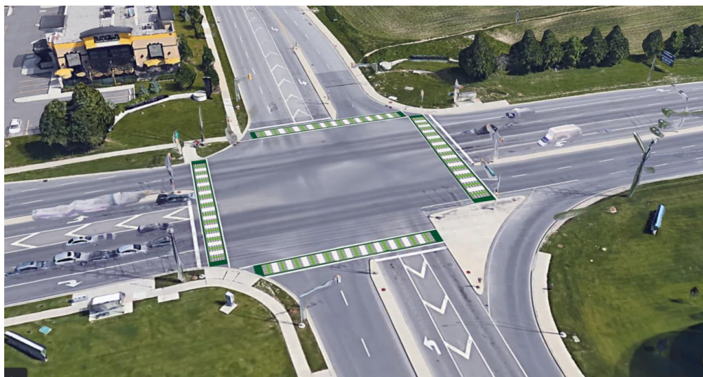
Diagram 2. Proposed crosswalk design
