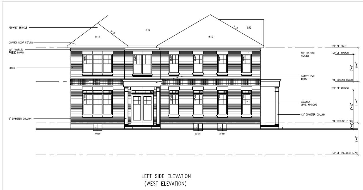
Figure 2: West elevation of the proposed replacement building.
