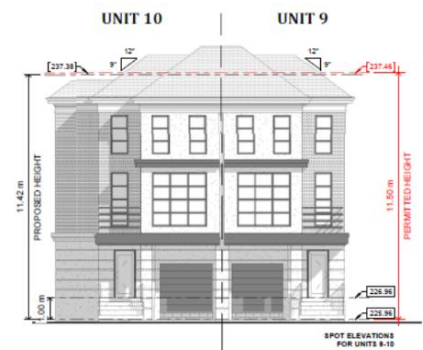
4 Unit 9-10 - Front Elevation - Height 1:100
