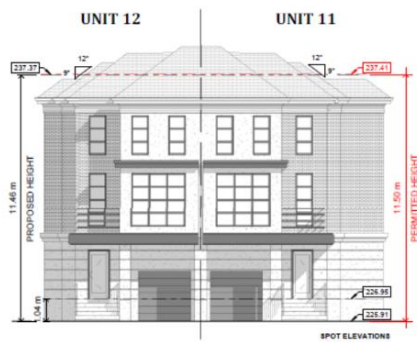
5 Unit 11-12 - Front Elevation - Height 1:100
