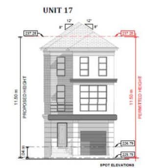
8 Unit 17 - Front Elevation - Height 1:100
