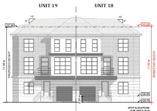
9 Unit 18-19 - Front Elevation - Height 1:100
