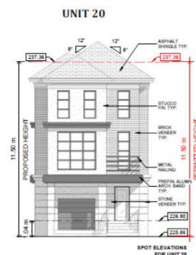
10 Unit 20 - Front Elevation - Height 1:100
