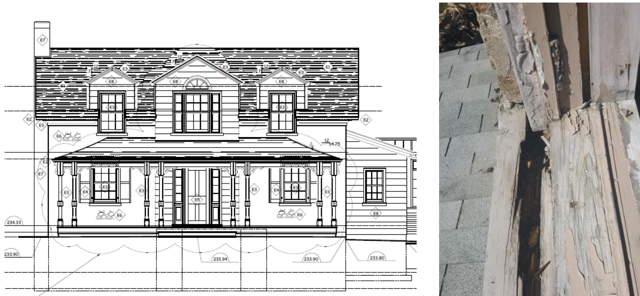
Figure 7 2021 Council-approved Heritage Permit drawing (left) showing the proposed east elevation of the Hilts House at 16 Bawden Dr. Note that the existing dormer windows are proposed to be replaced, and new historically appropriate ground-floor windows and door system are proposed to be installed. The photograph on the right shows the typical deteriorated condition of dormer window frames.
