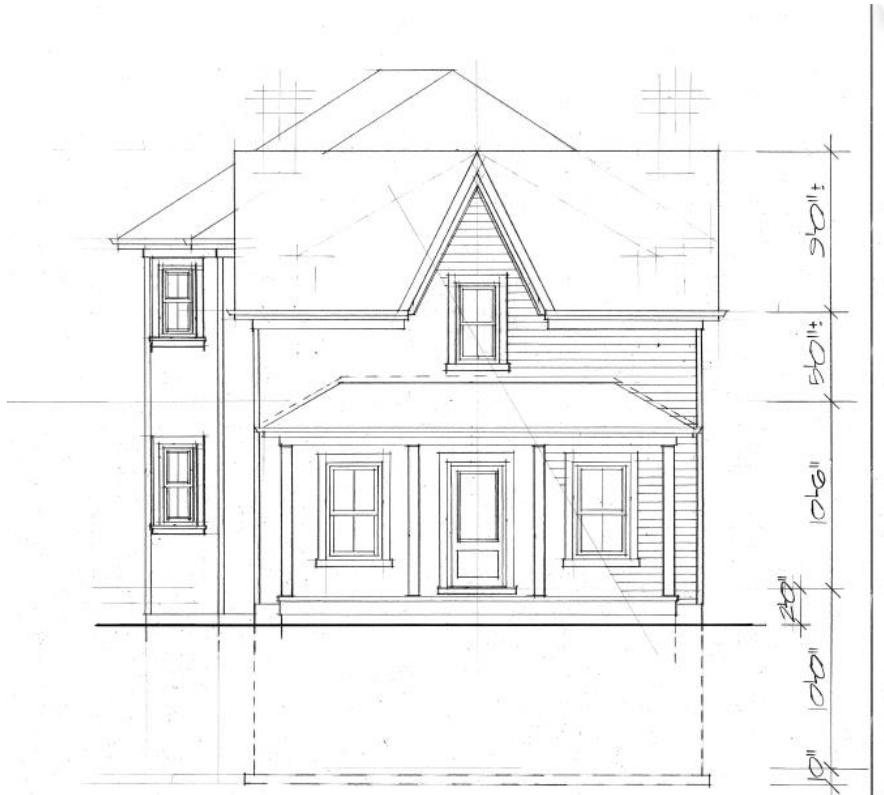
Figure 5 South elevation of the Eliza Gaby House, showing the conserved front portion of the house and the proposed rear addition (Source: The Gregory Design Group).
