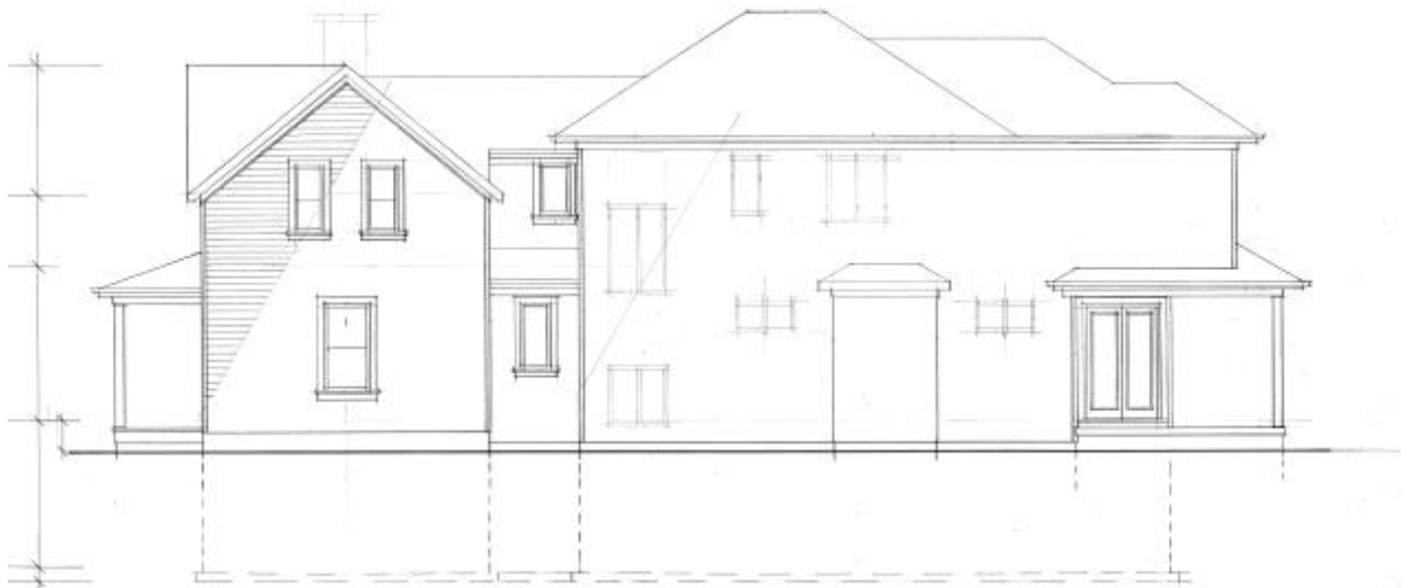
Figure 6 East elevation of the Eliza Gaby House, showing the conserved front portion of the house (left) and proposed rear addition (right) (Source: The Gregory Design Group).
