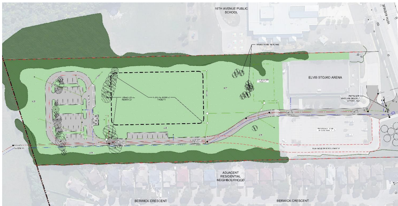
Figure 1: Site Servicing, Panhandle Access Road, Parking lot, Entrance Feature
