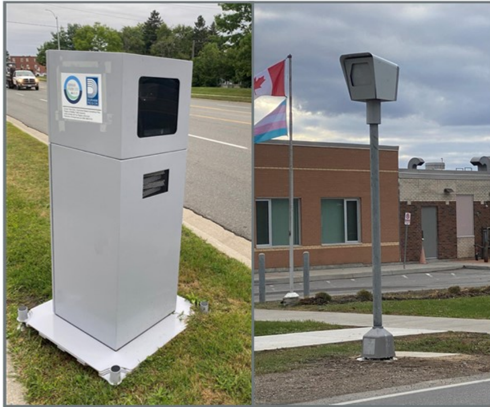
Figure 3-9 – Temporary (Left) and Permanent (Right) ASE Deployment 18
