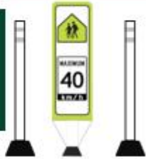
Flexible Bollards at School Crossing (East Leg)
