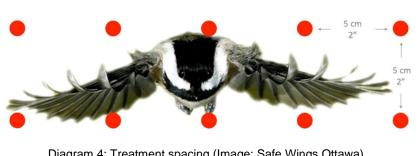
Diagram 4: Treatment spacing (Image: Safe Wings Ottawa)
