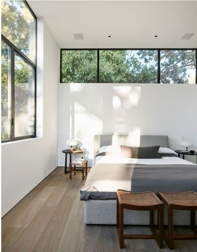
Figure 8. Clerestory windows in a bedroom. (Source: DigsDigs.com)
