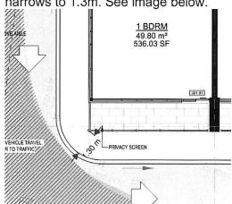
Pick-up / Drop-off areas should be conducted in a counter-clockwise maneuver to follow the proper direction of travel. Alternatively, the drive aisle must be one-way.
