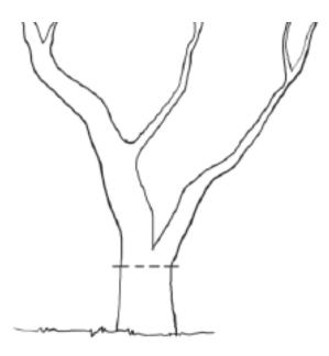
4. **Tree splits into several trunks close to ground level.** Measure DBH of each trunk separately, using the principles shown in categories 1-3 above. Square the DBH of all trunks. The DBH for the tree is found by taking the square root of the sum of all of the squared trunk DBHs.
