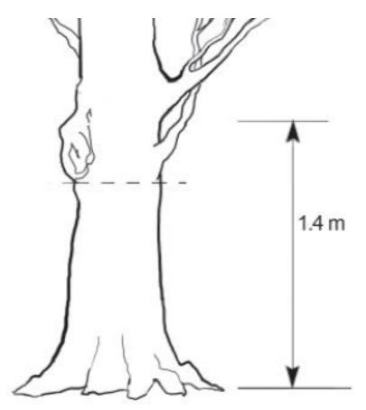
2. Vertically growing tree is on a slope or leaning tree. Measure diameter 1.4 m from the ground at the midpoint of the trunk parallel with the slope of the trunk.
