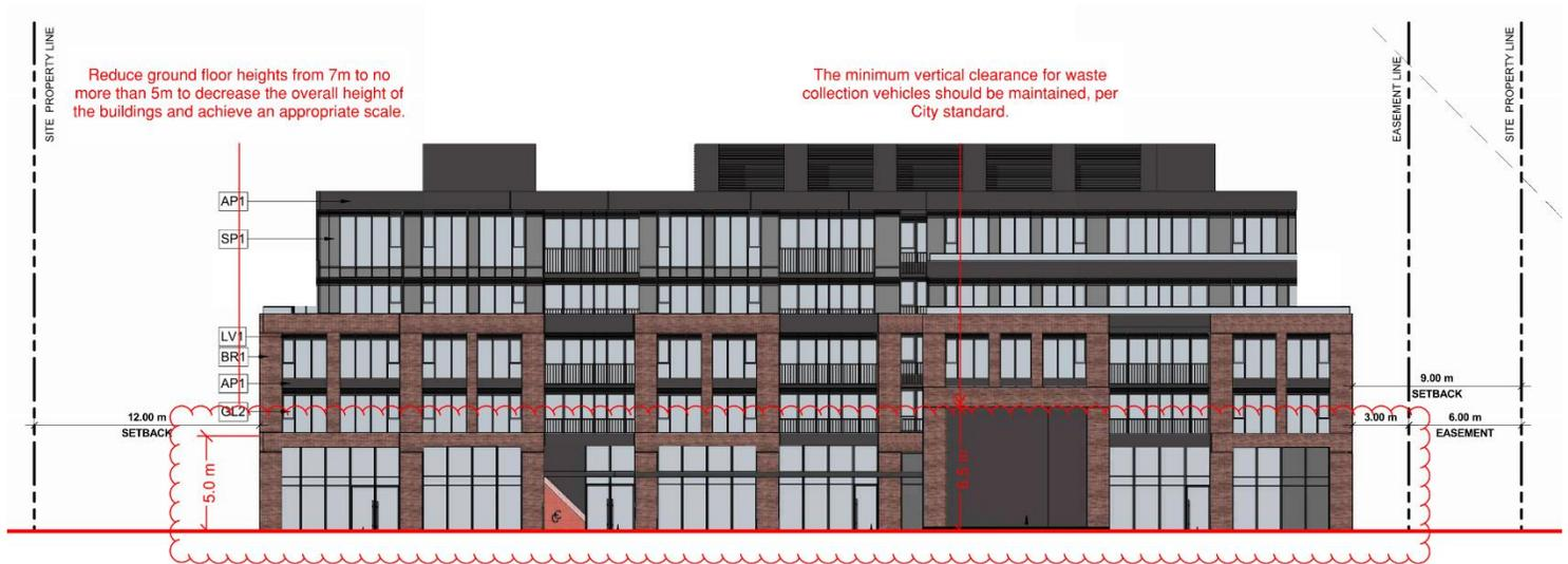
**Annotated Building 'A' South Elevation:** To decrease the overall height and achieve an appropriate scale, lower the ground floor heights of buildings from 7m to 5m; maintain the minimum required vertical clearance for waste collection vehicles.
